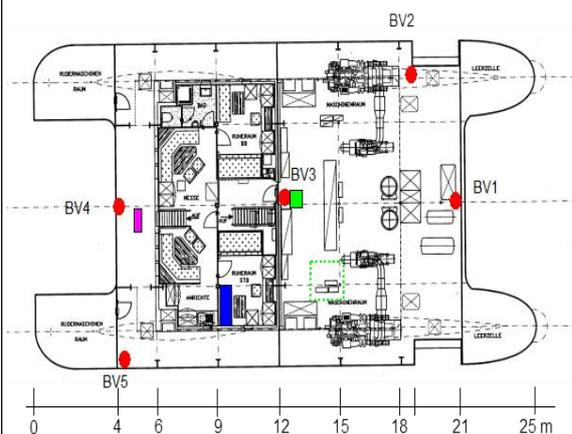
Accelerometers position on the main deck of the *Duhnen*.
